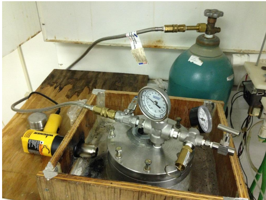
Figure A.4 Heating the vessel with a heat gun.
