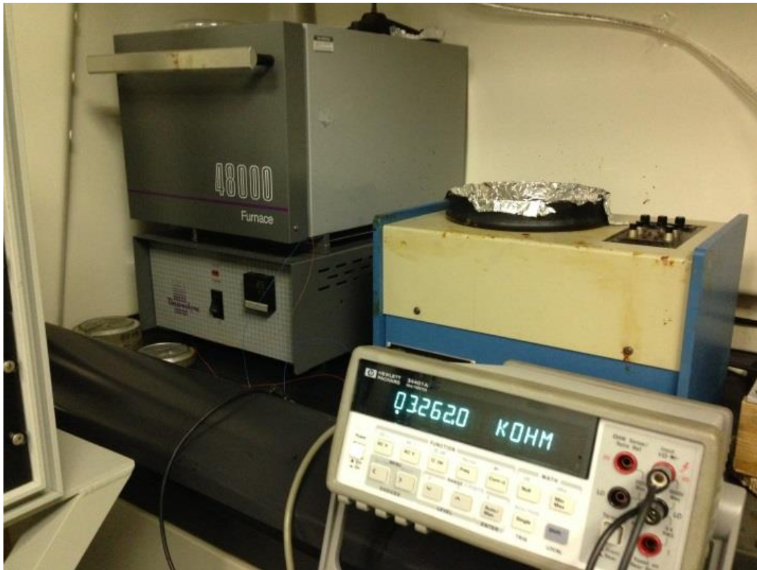
Figure 8.2 Measurement setup to determine TCR ( \alpha ).
