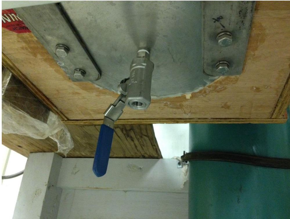
Figure A.3 Depressurizing or venting valve.
